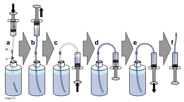
4. Couple the filled syringe to the inlet of the cooling circuit and press the cooling liquid inside the circuit. *Caution:* Position the empty bottle above the liquid circuit (on top of projector).
